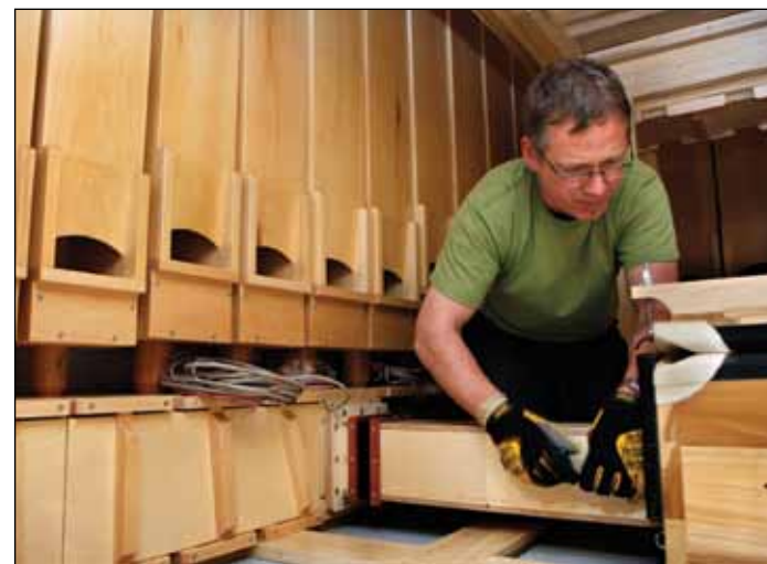
Thomas Rohlf of QLF fastens one of many wind conductors into place during the construction of the new Lively Fulcher organ at Community Church.
